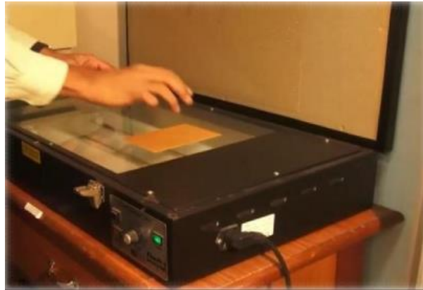
Fig. 12. The UV exposure unit
