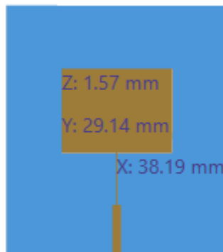
Fig. 17. Quarter-wavelength transformer diagram
