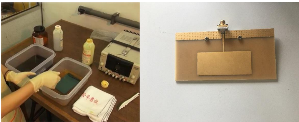
Fig. 13. Etching Process and last result RMPA produced
